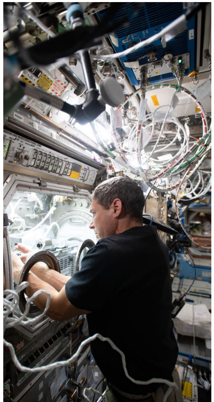
Astronaut and Engineer Michael Hopkins conducts research activities inside the Microgravity Science Glovebox.
