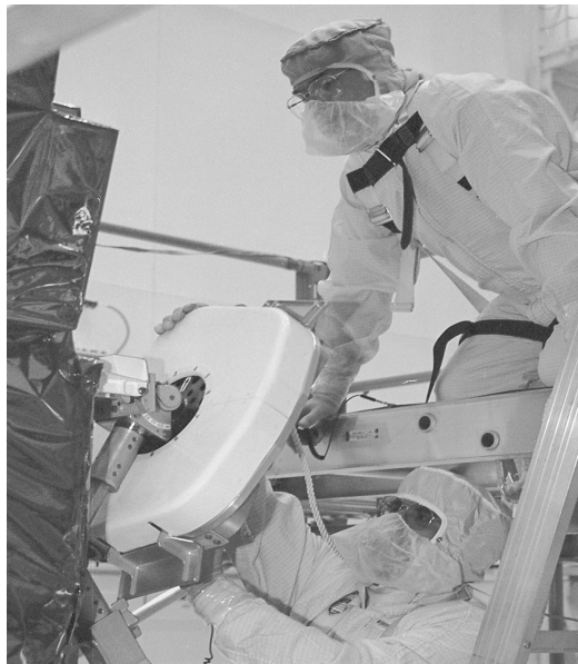
Technicians in Goddard's Clean Room install foot restraints on HST's Flight Support System.
