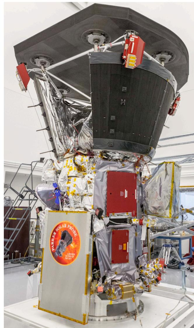
Parker Solar Probe Installation of the Flight Thermal Protection System at APL, Sep 21
