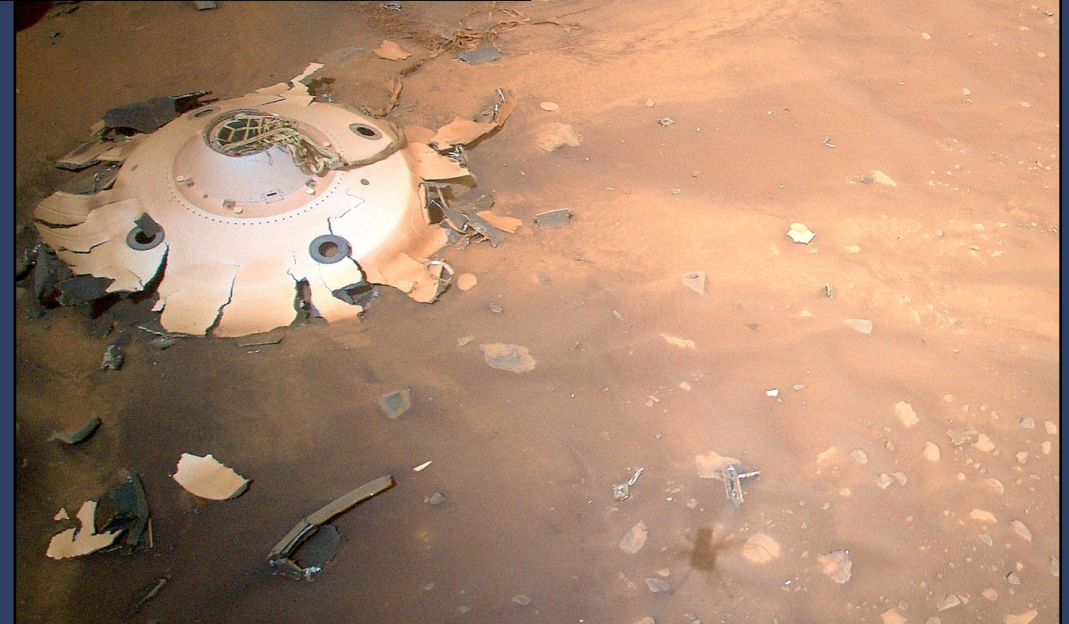
This image of Perseverance's backshell and supersonic parachute was captured by NASA's Ingenuity Mars Helicopter during its 26th flight on Mars on April 19, 2022. Credit: NASA/JPL-Caltech
