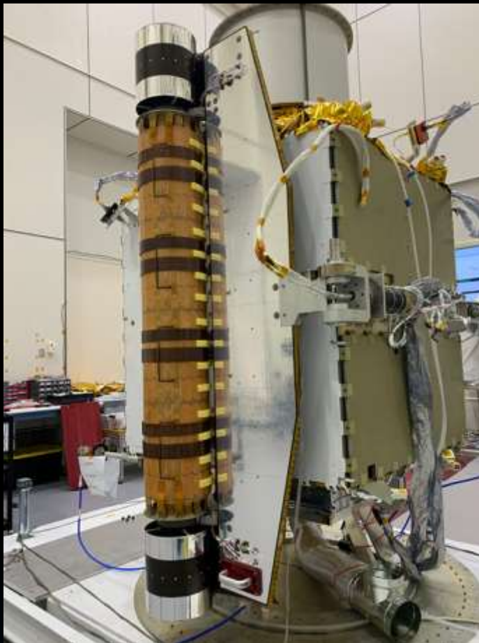
ROSA Wing 1 Installed on Spacecraft
