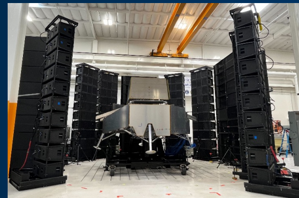
Astrobotic Griffin lander STM; acoustic testing
