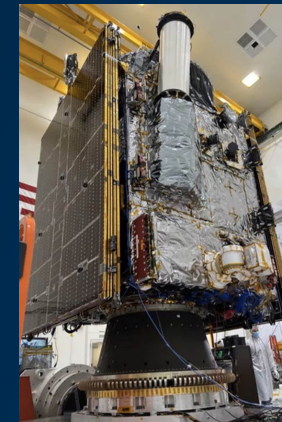
Psyche on shaker table for dynamics testing
