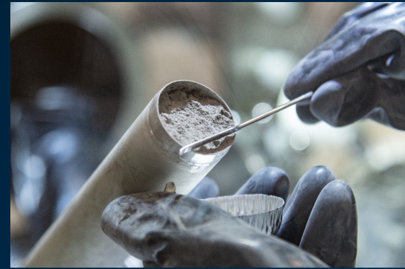
ANGSA: Apollo 17 lunar core sample 73001 being taken out of its drive tube for the first time since 1972
