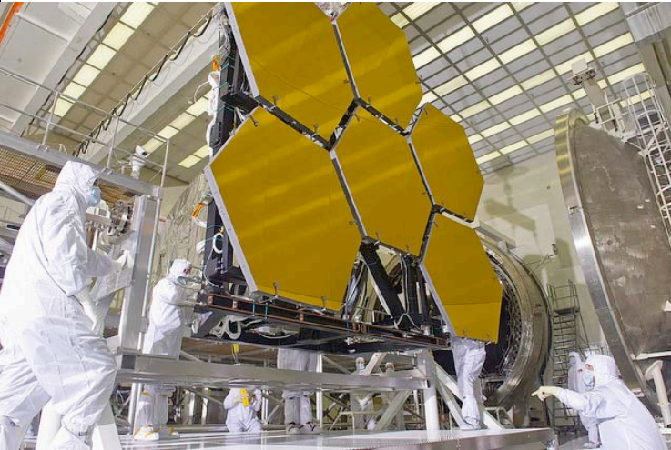
Final Set of Mirrors at the XRCF
