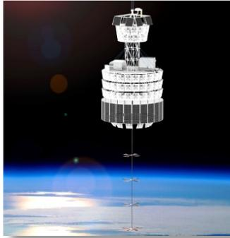
**PUEO:** A Long-duration Balloon-borne Instrument for Particle Astrophysics at the Highest Energies,
