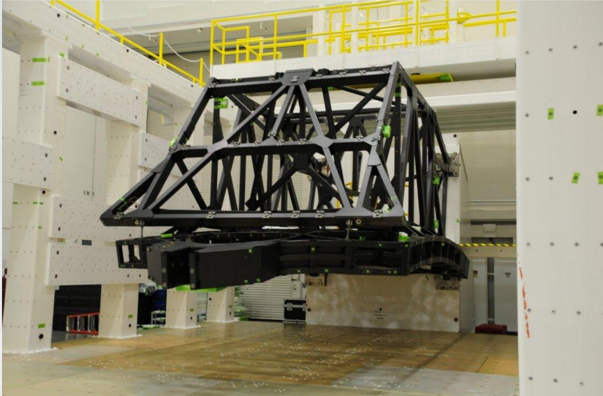
Backplane Center Section & Backplane Support Fixture at NGAS for Static Loads Testing Completed Wing backplanes being tested at ATK, Secondary Mirror Mount delivered to NGAS
