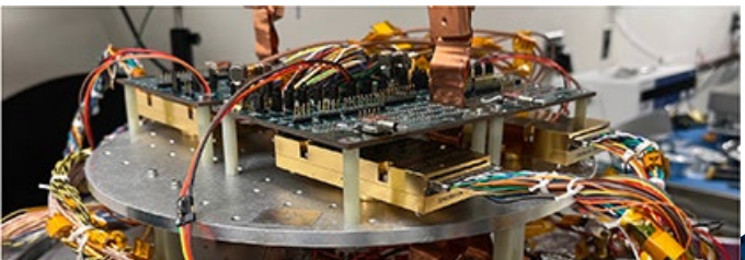
First 4 Flight Sensor Control Electronics (SCE) installed and undergoing functional test
