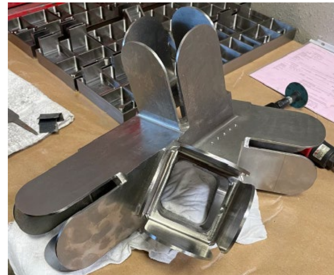
Instrument Carrier Upper Assembly Titanium Fitting - fabrication nearly complete
