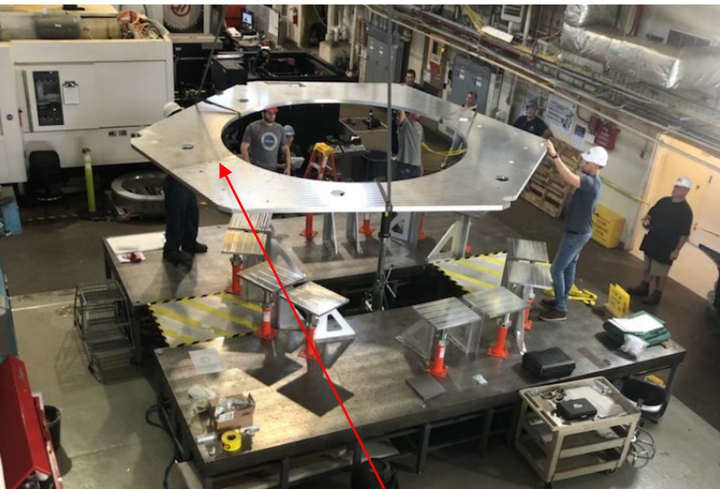
Bottom deck (above), Central cylinder (top right), and Top deck (lower right) in B.5 high bay for Spacecraft Bus assembly
