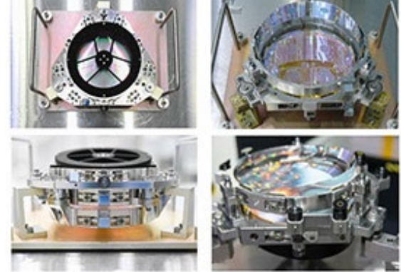
Flight Filters, Grism and Prism complete; installed and aligned in EWA
