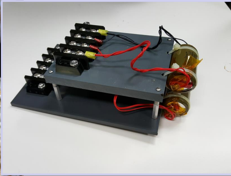
Test fixture used during irradiation of primary battery cells
