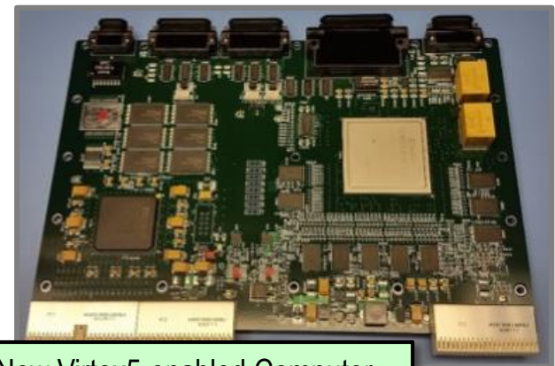
New Virtex5-enabled Computer Vision Accelerator Card (CVAC)
