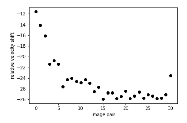
Calibrated instrumental stability with LFC – RMS ~ 5 cm/s over 10 hours.
