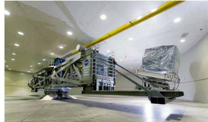
ISIM flight structure ambient temp strength testing
