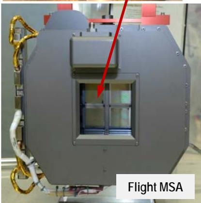
203 x 463 mas shutter pixel clear aperture, 267 x 528 mas pitch, 4 x 171 x 365 array
