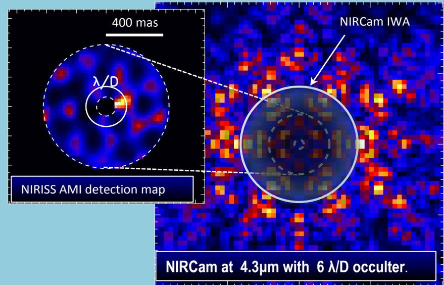
Simulated companion above has contrast of 10 mag at a separation of 130 mas
