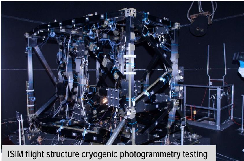
ISIM flight structure cryogenic photogrammetry testing
