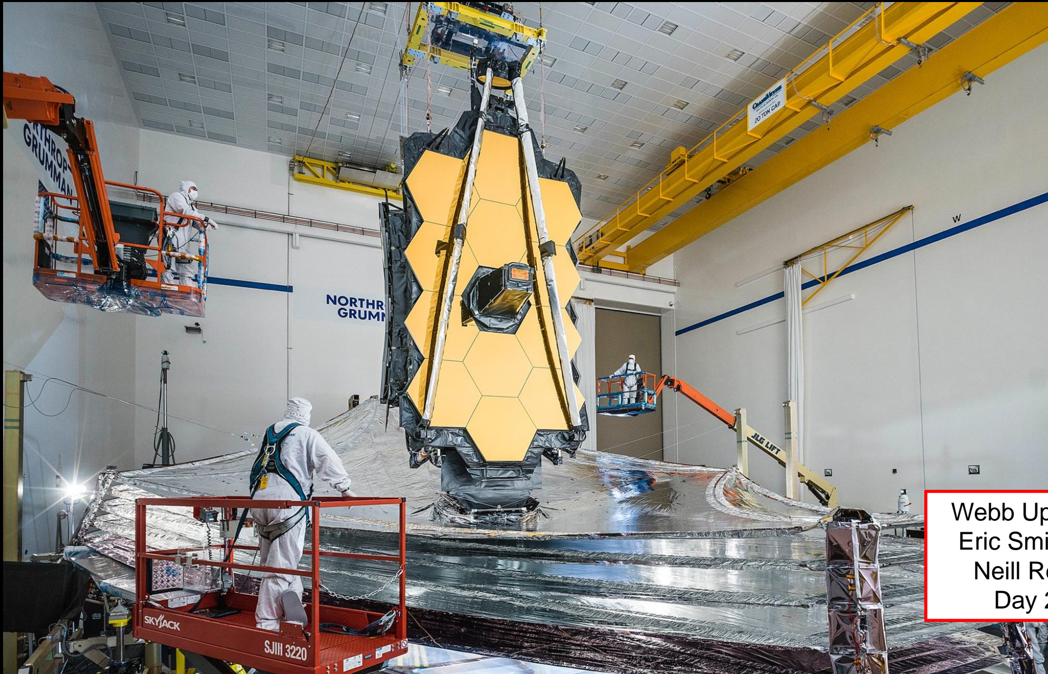
The final deployment of Webb's sunshield on Earth (Northrop Grumman Space Park, December 2020). Webb will undergo folding and stowing before shipment and mating to the Ariane 5 in 2021.
