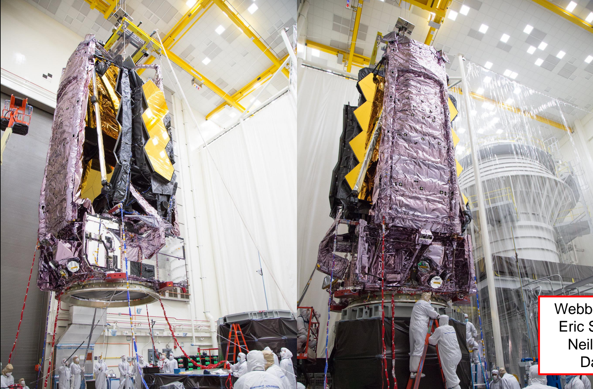
The fully assembled and folded James Webb Space Telescope on the vibration table at Northrop Grumman Space Park (September 2020). This is the configuration that Webb will be in when it is mated to the Ariane 5 launch vehicle in 2021.
