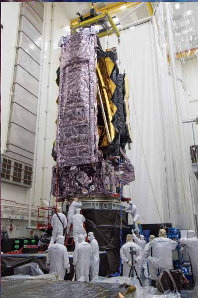
The Webb observatory on the vibration table in Redondo Beach, CA in September 2020
