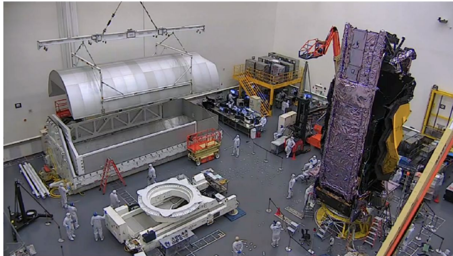
Shipping container, roll-over fixture and Webb at Northrop Grumman
