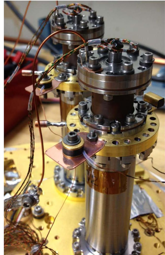
Flight Model Heat Switches being prepared for functional testing
