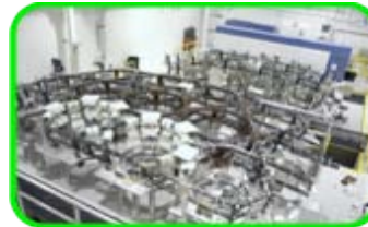
Primary Mirror Support Structure
