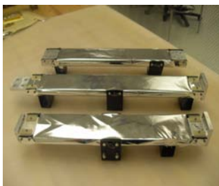
Flight high purity aluminum heat strap assemblies
