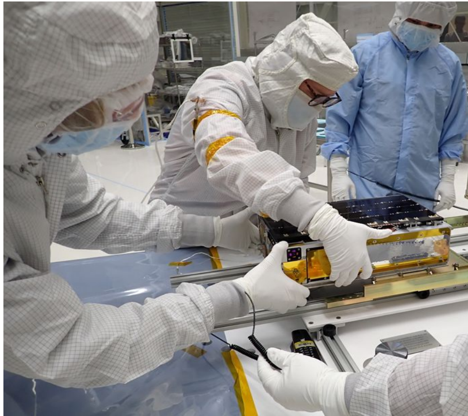
Grad Student Arika Egan (center) and PM Nick DeCicco (left) insert CUTE in launch deployment canister at VAFB. Photo courtesy K. France
