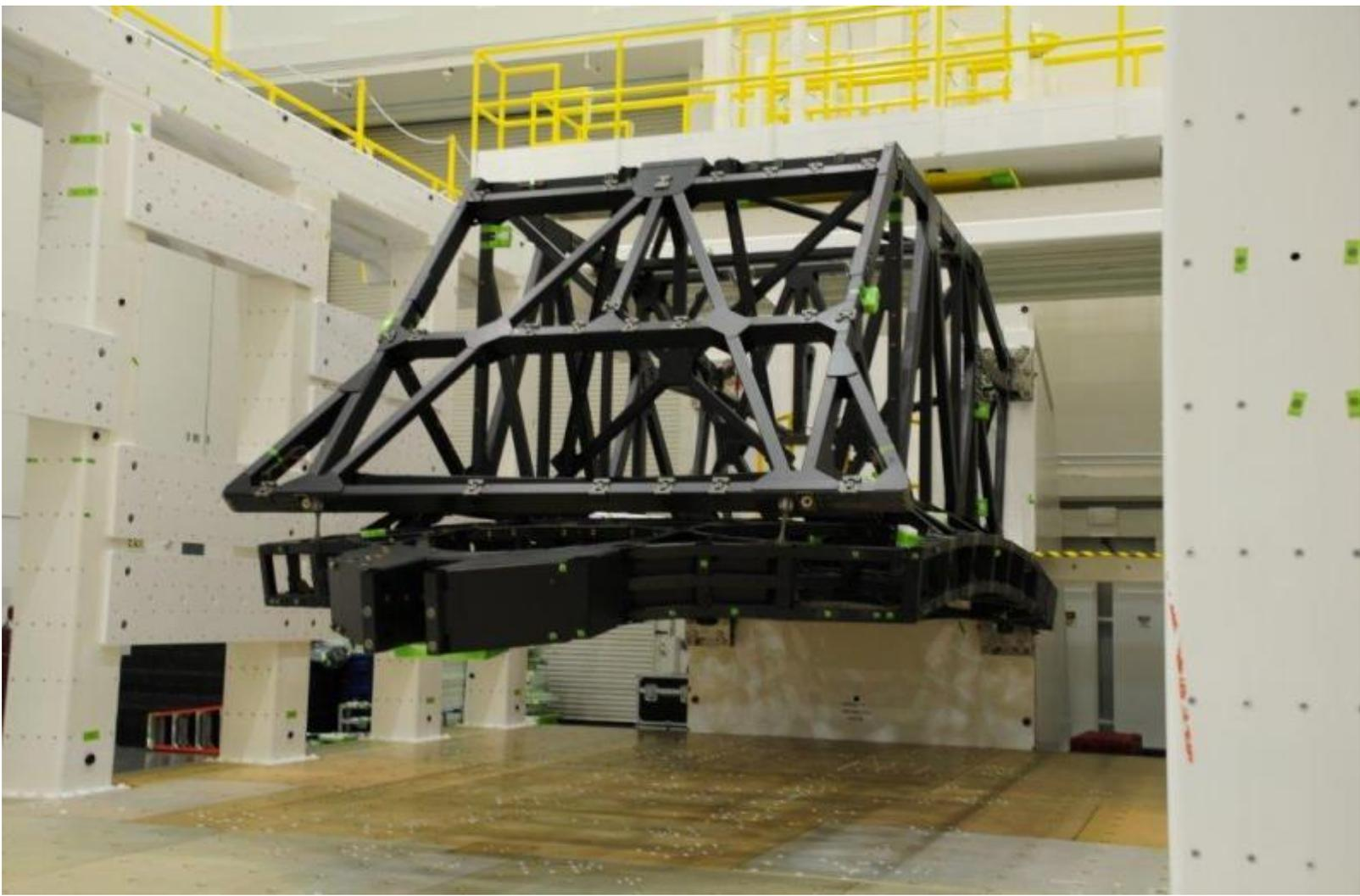
Flight Backplane Suspended from Strong Back in Load Test Fixture at NGAS
