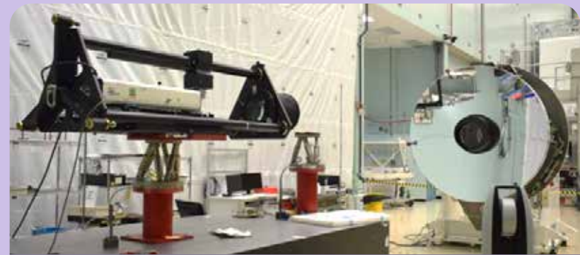
Primary Mirror horizontal optical test
