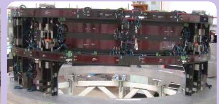
Forward Metering Shell w/thermal control hardware installed
