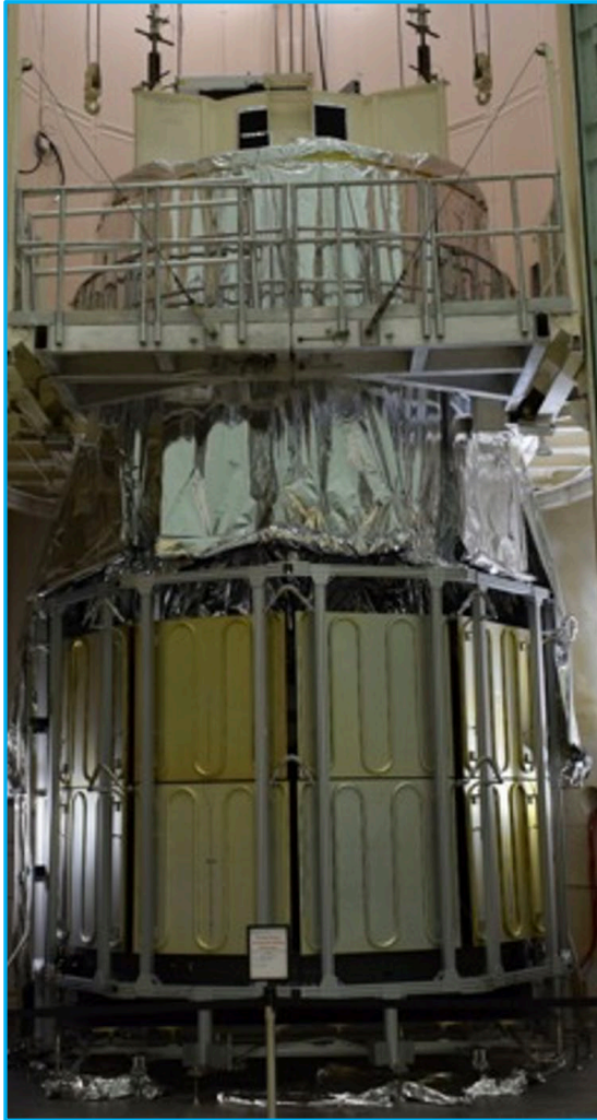
Primary Mirror Assembly in Chamber IIIA with shrouds in place
