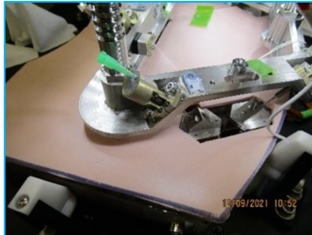
Fold Mirror 2 Assembly Stycast Operation
