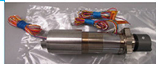
Flight gear motor for Element Wheel Assembly received at Ball and in-process for integration
