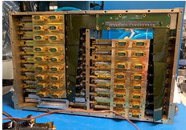
Focal Plane Electronics Engineering Test Unit in final assembly
