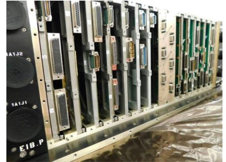
Telescope Control Electronics (TCE) Module Complete
