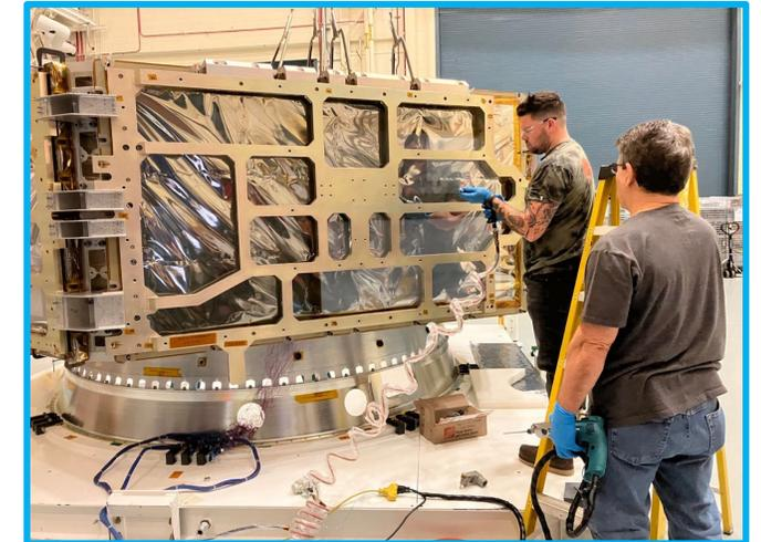
Match drilling of bus to avionics panels in B.29 High Bay
