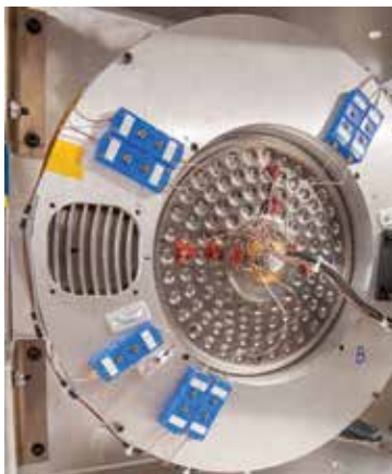
The Radial Core Heat Spreader shown mounted inside the experiment heat exchanger during preparations for the suborbital flight test.
