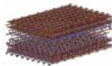
A multi-layer weave schematic showing high-density top and bottom layers with a mid-density layer with different yarn composition.
