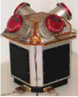
This cluster of four colloid thrusters is part of the Disturbance Reduction System, developed by NASA/JPL, which will help keep the LISA Pathfinder spacecraft extremely stable. (Image credit: ESA/NASA/JPL-Caltech)
