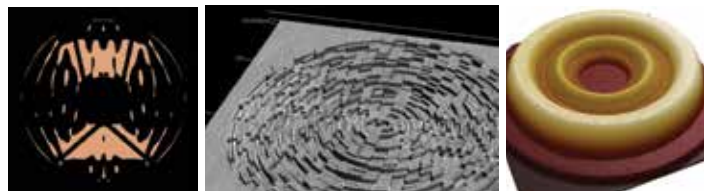
Pupil-plane reflective mask for the SPC, 24-mm diameter, black silicon on mirror (left). Image-plane reflective mask for the back-up technology Phase Induced Amplitude Apodization Complex Mask Coronagraph (PIAA-CMC) coronagraph, 155- \mu m diameter, raised elements on silicon (center). Image-plane transmitting mask for HLC, 100- \mu m diameter, raised dielectric and metal on glass (right). All masks were fabricated in the Micro-Devices Lab (MDL) at the Jet Propulsion Laboratory (JPL).
