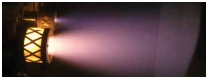
Busek's 65W iodine-fueled ion propulsion system "BIT-3," currently scheduled to fly on the LunaH-Map and Lunar IceCube missions.
