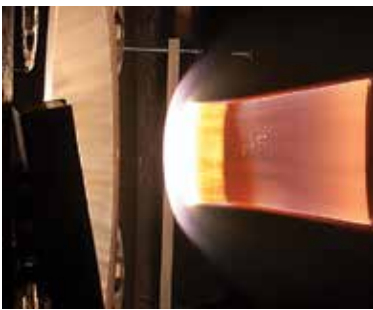
Testing of HEET material at the NASA Ames Arc Jet Complex in the Interaction Heating Facility.
