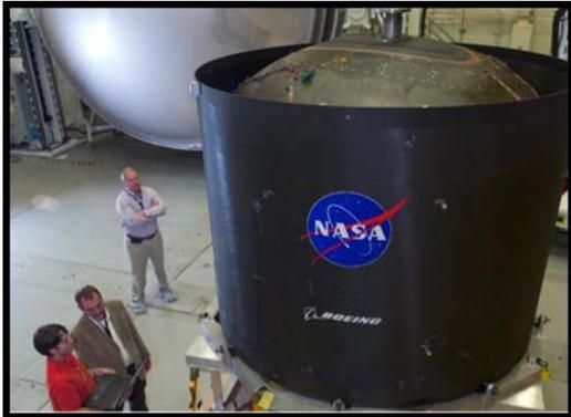
Arrival and testing of 2.4m precursor tank, the largest out-of-autoclave tank fabricated in the world
