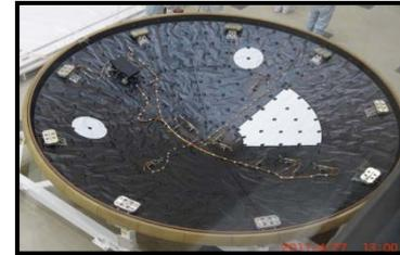
**MSL Heat Shield with Instrumentation**
