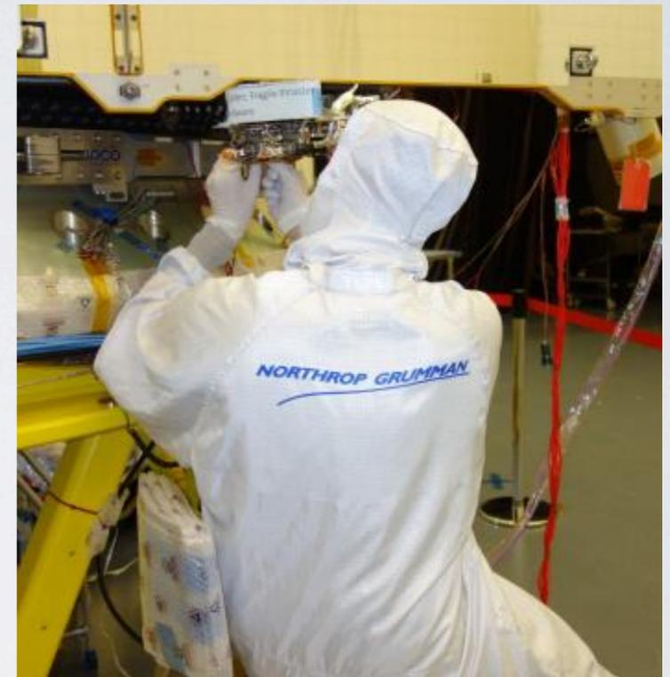
Technician works on easily accessible Thruster Assembly
