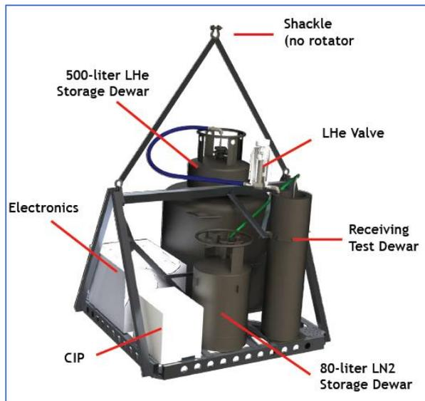
**BOBCAT** - (Kogut/GSFC) develops technology to improve far-IR sensitivity by a factor of 1000,000 compared to ground-based facilities or SOFIA. BOBCAT-1 is a technology demo of liquid nitrogen and liquid helium cryogen transfer. BOBCAT-2 is a demo of ultra-light balloon dewars.
