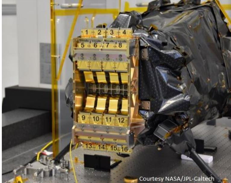
Near Infrared Spectrometer and Photometer - fully populated focal plane includes NASA provided 16 (2K x 2K each) Sensor Chip Systems
