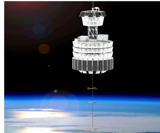
Figure 10: A rendering of the PUEO payload, including a design for the low-frequency drop-down instrument.
