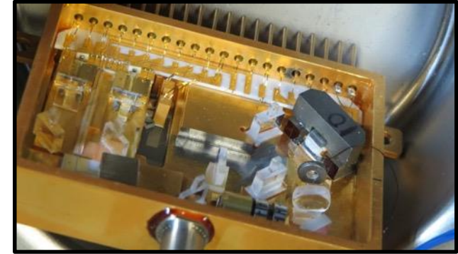
(top) mNPRO master oscillator under test at GSFC. (bottom left) Fiber amplifier. (bottom right) frequency reference cavity for GRACE-FO.
