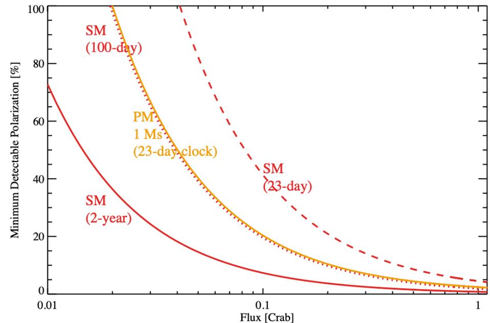
Polarization sensitivities for Survey Mode (SM) vs. Pointed Mode (PM)
