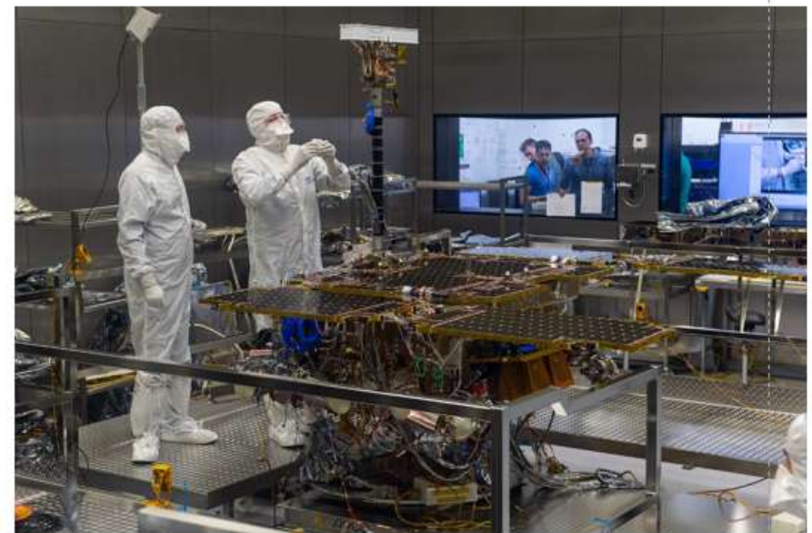
Pancam Integration in Rover FM
