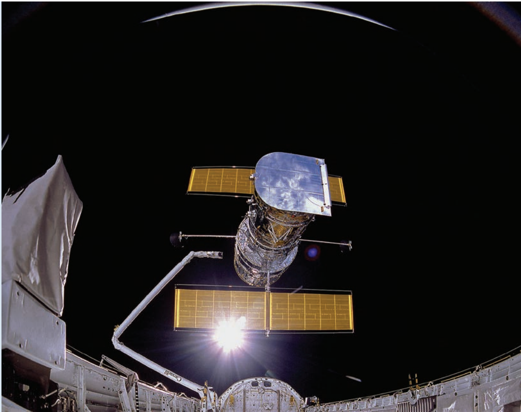
▲ An IMAX camera in the rear of Discovery’s payload bay obtained this image of the Hubble Space Telescope moments after its release into space by the Space Shuttle Remote Manipulator System on 25 April 1990 during the STS-31 mission. (NASA: 9015550)
