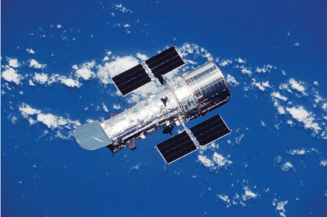
▲ The Hubble Space Telescope (HST) returns to its normal observing routine after a week of servicing and upgrading by the STS-109 astronaut crew aboard the Space Shuttle Columbia in March 2002. Following that mission, HST was equipped with its third set of solar arrays, which are smaller than the first two sets. (NASA: STS109-331-010)
