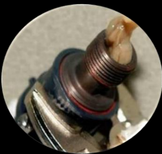
Russian condensate processor biofilm. Image provided by NASA.
