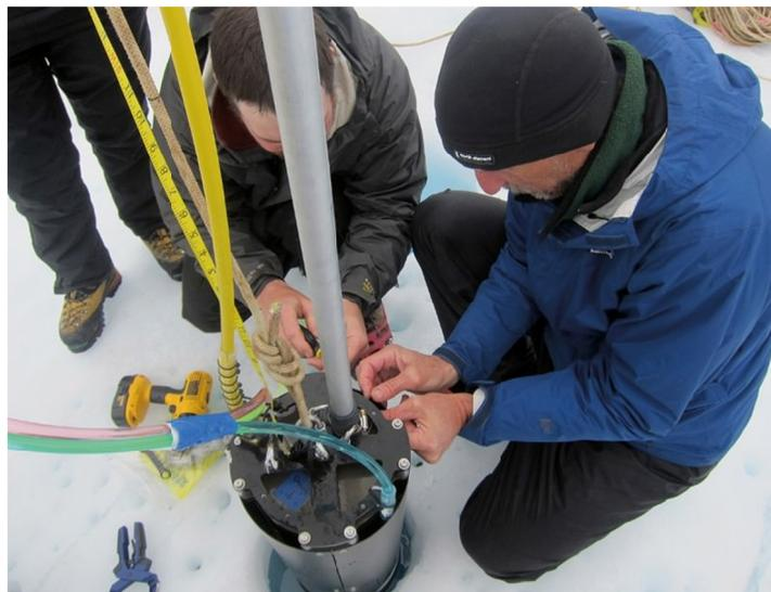
FIGURE 4.3 Scientists conduct field tests for the NASA funded robotic explorer VALKYRIE (Very-deep Autonomous Laser-powered Kilowatt-class Yo-yoing Robotic Ice Explorer), created by Stone Aerospace on Matanuska glacier in Alaska as an analogue for Europa. VALYRIE was funded via a predecessor of the current Planetary Science and Technology Through Analog Research program element for field testing of mid-technology readiness level instrumentation in analogue environments on Earth.
