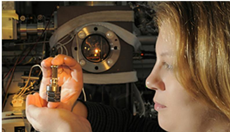
FIGURE 1.2 A NASA scientist holds a piece of the sensor for the Linear Ion Trap Mass Spectrometer, a highly compact mass spectrometer funded under the MatISSE (Maturation of Instruments for Solar System Exploration) program. SOURCE: Pat Izzo/NASA.
