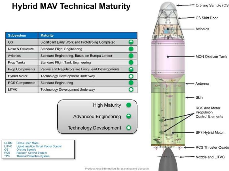
FIGURE 5.11 Schematic image of the Mars Ascent Vehicle (MAV) currently under study. MAV technology is finally making substantive progress. SOURCE: JPL.
