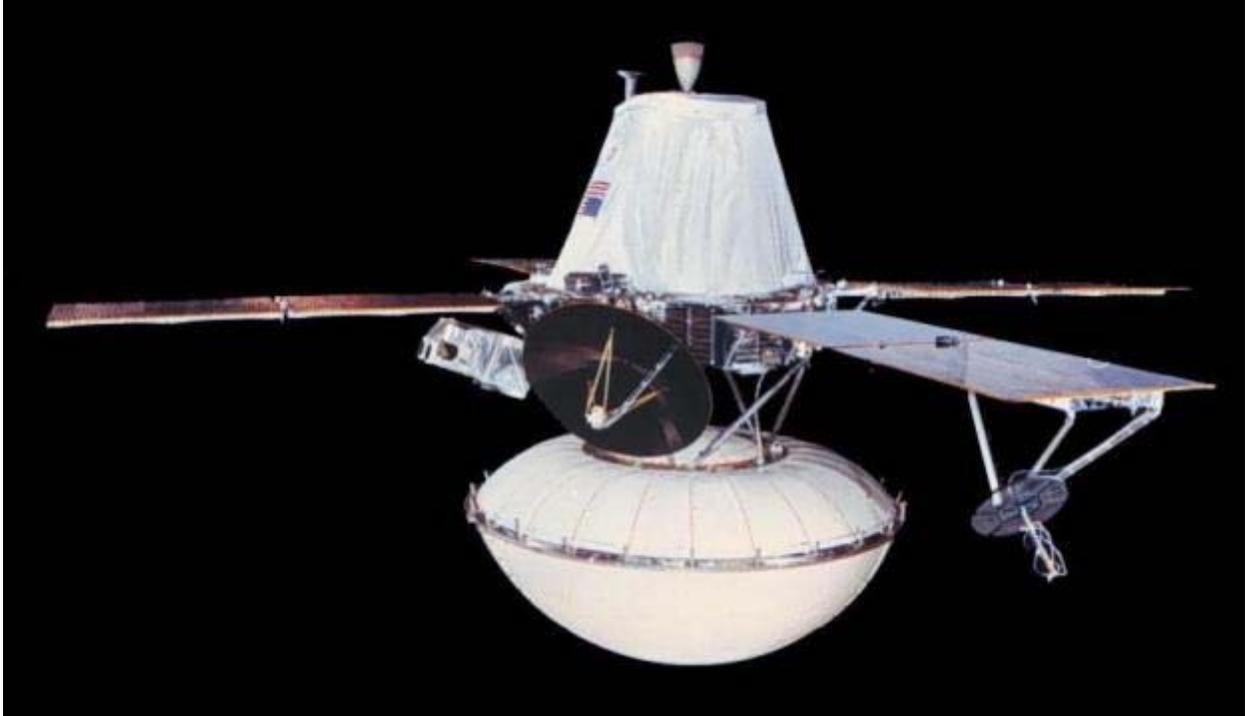
FIGURE 5.1 Mockup of the Viking spacecraft, which consisted of both an orbiter and a lander. SOURCE: NASA/JPL.
