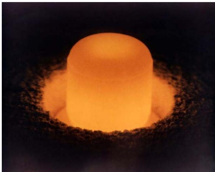
FIGURE 4.1 Pellet of Pu-238 for RTG use. SOURCE: The Planetary Society, “Plutonium-238 Fuel Pellet,” <http://www.planetary.org/multimedia/space-images/spacecraft/plutonium-238-fuel-pellet.html>; courtesy of the U.S. Department of Energy.
