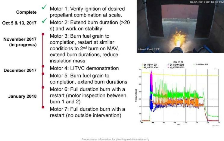
FIGURE 5.12 Test of one of the MAV hybrid rocket motor engines in fall 2017. SOURCE: JPL.
