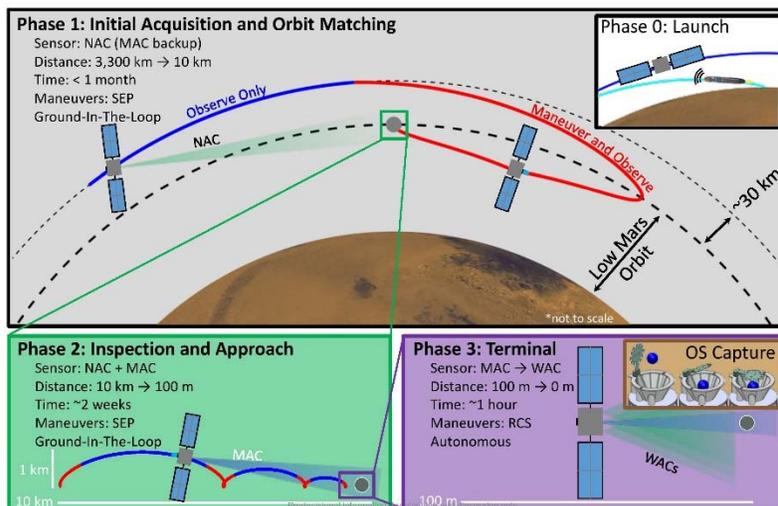
FIGURE 5.16 Rendezvous concept for the Orbiting Sample vehicle that would carry samples collected by the Mars 2020 rover. SOURCE: JPL.
