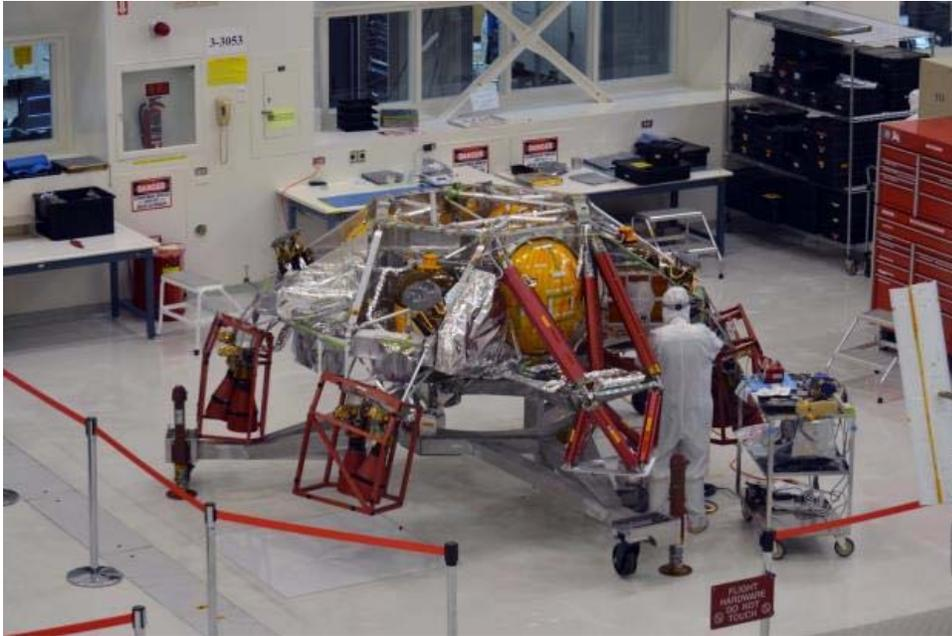
FIGURE 1.6 Construction work on descent stage for Mars 2020. The Mars 2020 spacecraft is heavily based on the successful Mars Science Laboratory/Curiosity rover mission that landed on Mars in 2012. SOURCE: NASA Jet Propulsion Laboratory, “JPL Tech Works Mars 2020 Descent Stage,” PIA22342, courtesy of NASA/JPL-Caltech.
