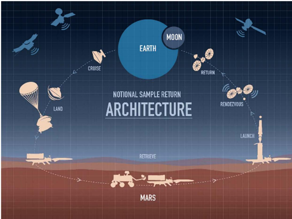
FIGURE 5.10 Notional concept image for implementation of the two future missions required to complete Mars Sample Return, a Fetch Rover and Mars Ascent Vehicle, and a Sample Return Orbiter. SOURCE: NASA.
