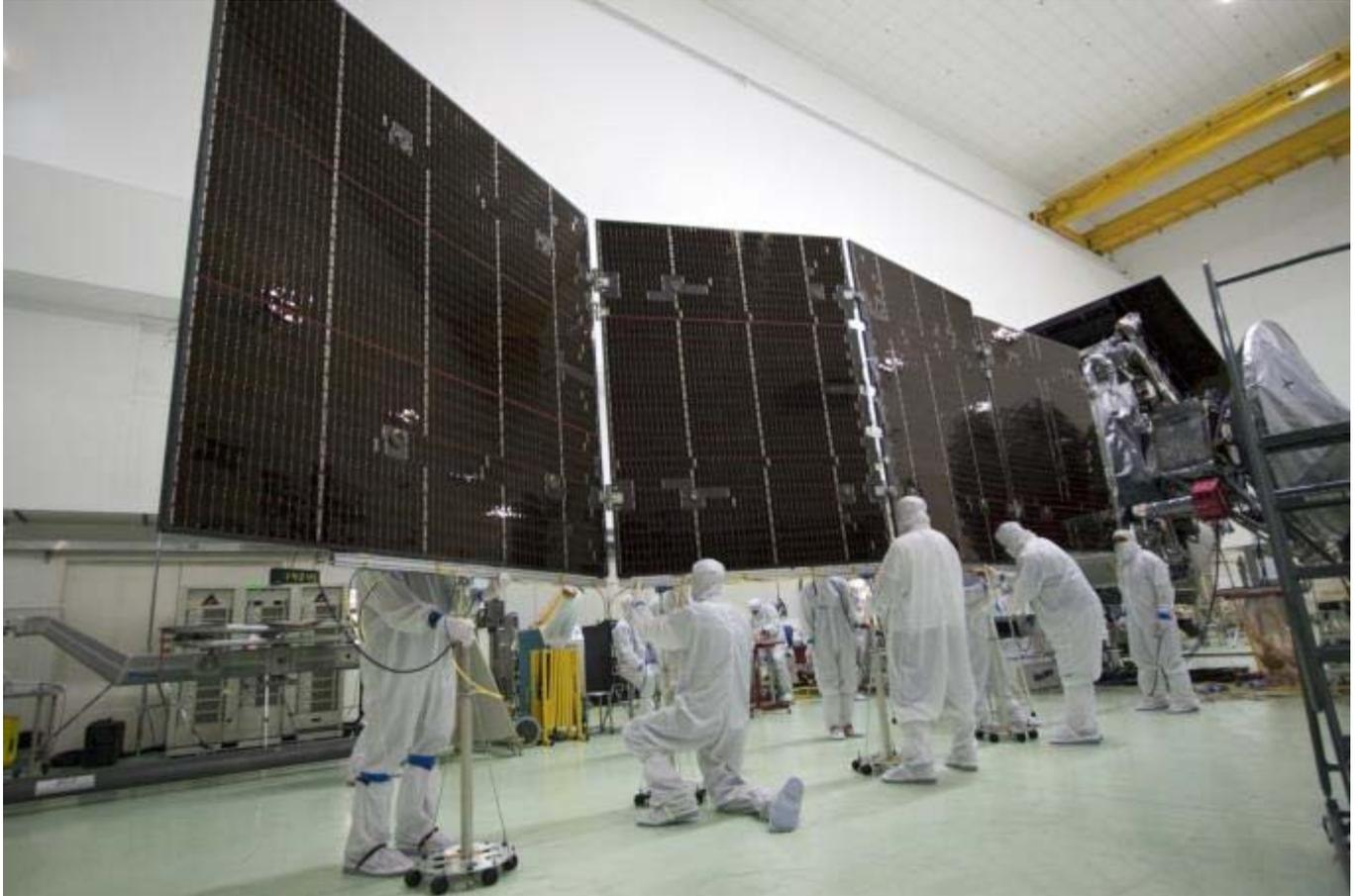
FIGURE 1.3 The Juno spacecraft with solar array arm outstretched in testing. Juno began orbiting Jupiter in 2016. In addition to making new scientific discoveries, Juno has demonstrated the use of solar power at Jupiter distances from the Sun. SOURCE: NASA, “Packing Juno’s Power,” PIA14172, <https://photojournal.jpl.nasa.gov/>; courtesy of NASA/JPL-Caltech/KSC.
