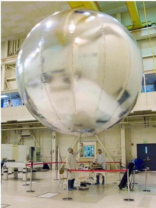
FIGURE 4.5 Testing of a balloon concept for the Venus Climate Mission. SOURCE: NASA.
