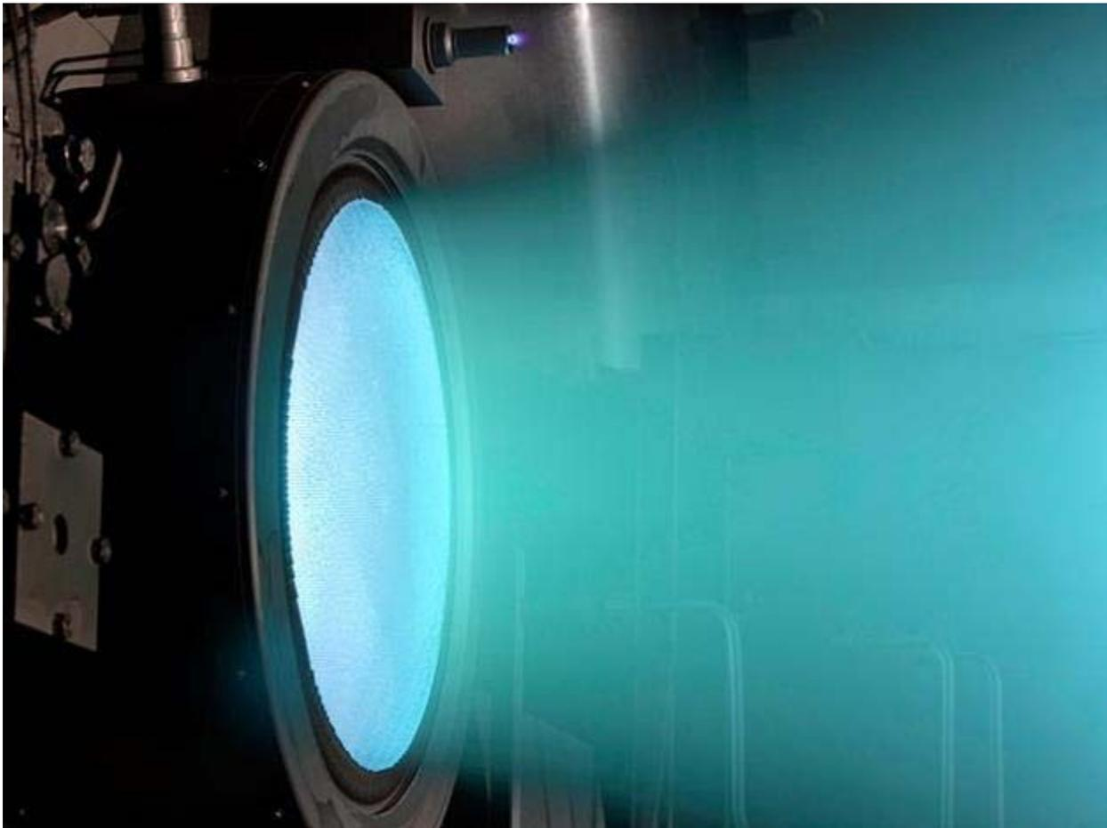
FIGURE 4.3 NEXT-C ion thruster during test. SOURCE: NASA Glenn Research Center, “NASA’s Evolutionary Xenon Thruster (NEXT) Project has developed a 7-kilowatt ion thruster for deep space missions,” <https://www1.grc.nasa.gov/facilities/epl/>.
