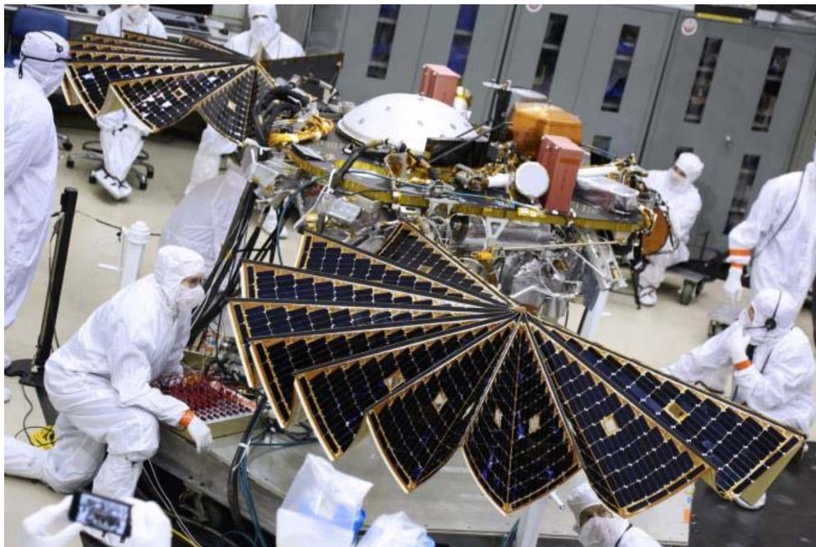
FIGURE 3.7 InSight with wings out for solar array test. SOURCE: NASA, “InSight Lander Solar Array Test,” January 23, 2018, <https://mars.nasa.gov/insight/multimedia/images/2018/insight-lander-solar-array-test>; courtesy of Lockheed Martin Space.
