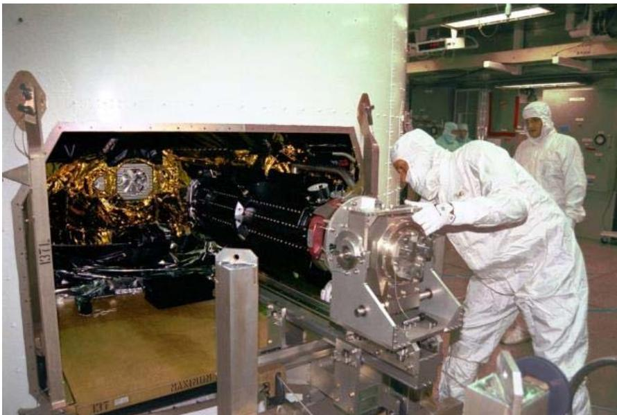
FIGURE 1.9 Beginning the Radioisotope Thermoelectric Generator (RTG) installation for Cassini. Pu-238 production for RTGs ceased in the 1980s and is only now being restarted. SOURCE: NASA JPL,
