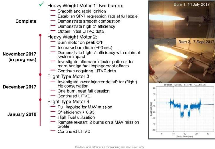
FIGURE 5.13 Test of one of the MAV hybrid rocket motor engines in fall 2017. SOURCE: JPL.
