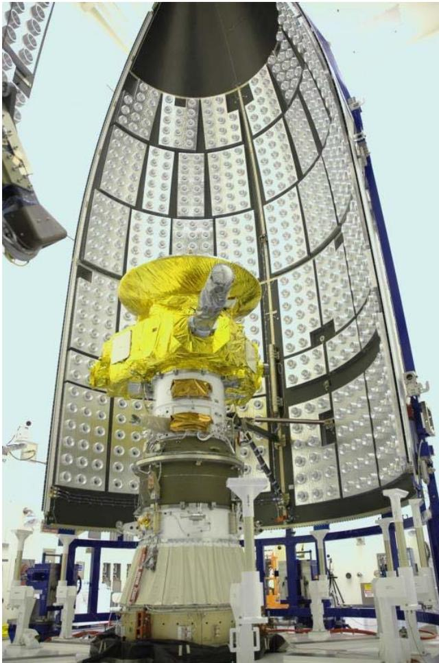
FIGURE 1.2 New Horizons being placed into its launch shroud. The spacecraft flew past Pluto in summer 2015, returning data that revealed Pluto to be a complex world in the far reaches of our solar system. SOURCE: NASA Kennedy Space Center, <https://mediaarchive.ksc.nasa.gov/#/Image/4980/S>.
