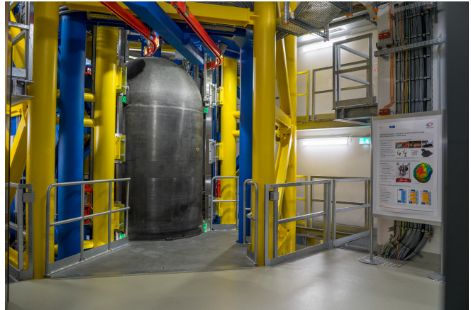
FIG. 1. Start position of the Einstein-Elevator for a vertical parabolic flight (credit: Leibniz University Hannover/Marie-Luise Kolb, licence: CC-BY 3.0 DE, [29]).
