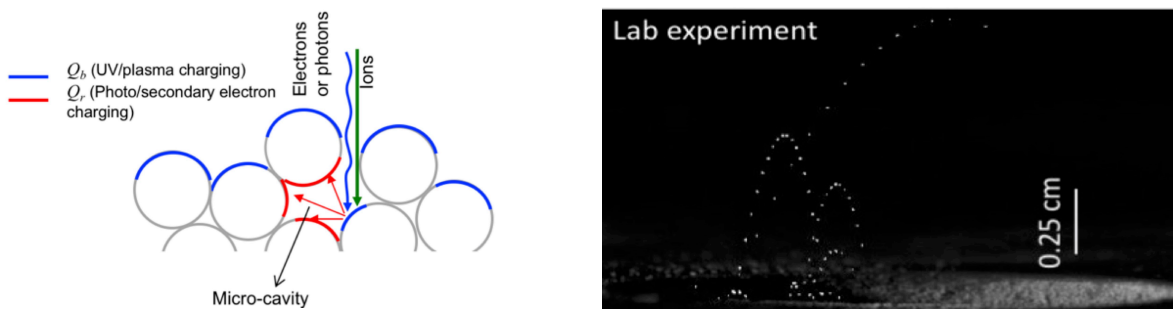
Fig. 3 Left : Patched Charge Model for regolith dust particles [Wang et al., 2016]; and Right : Trajectories of electrostatically lofted dust particles [Wang et al., 2016].
