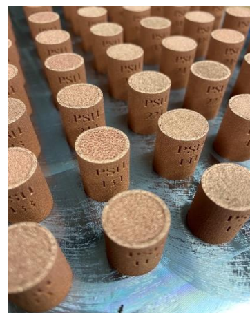
Figure 1. Copper porous samples fabricated by additive manufacturing.
