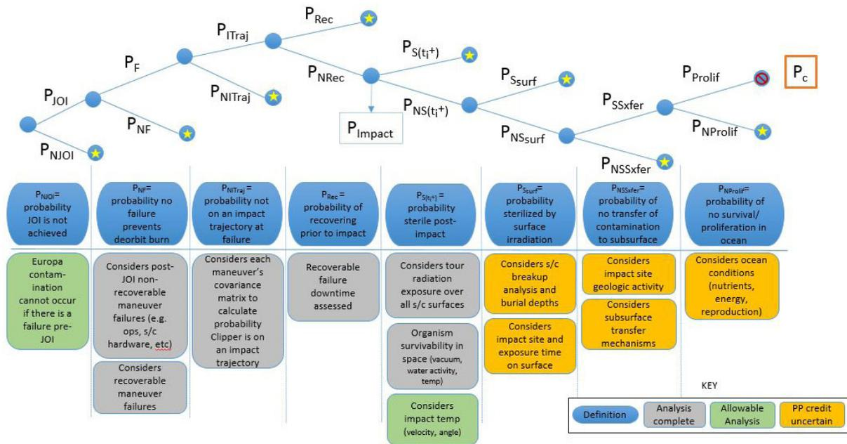
**FIGURE 3.6** A schematic depiction of the Icy Bodies Planetary Protection Probabilistic Model used to calculate the probability of icy body contamination. SOURCE: Redrafted from an original provided by the Europa Clipper Project, NASA, Jet Propulsion Laboratory
