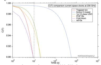
Clock coherence vs. time at a detection frequency of 230 GHz for current space clocks showing a distinct difference between the maser and all others. A value of nearly 1 is required for VLBI – less than one indicates coherence loss. The dashed vertical line is at 10 s, the approximate requirement for EHT observations.
