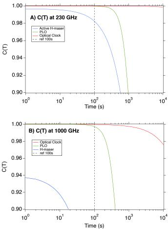
Comparison of clock coherence vs. time with a detection frequency of a) 230 GHz and b) 1000 GHz for emerging optical clock technologies (not yet operating in space.) The active H-maser is included for comparison. A value near 1 is required for VLBI. The dashed black line is at 100 s, a desirable SVLBI coherence time.
