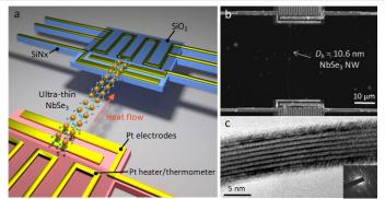
Figure 1: (a) Schematic illustration of the measurement device with a NbSe<sub>3</sub> nanowire placed between the heat source and heat sink. (b) An SEM micrograph showing a nanowire on the device with a suspended length of 28.2 um. (c) An HRTEM image of an ultra-thin NbSe<sub>3</sub> nanowire showing the crystalline structure.
