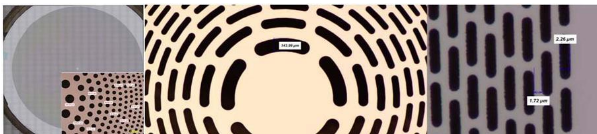
Figure 8. Photon sieves photolithographically fabricated in silicon wafers at GSFC. Left: photograph of an 80-mm diameter sieve with 1,666 zones comprising 17,591,294 holes ranging in size from 290 \mu\text{m} to 7 \mu\text{m} in diameter. Left Inset: micrograph of innermost zones. Center and right: micrographs of the center and edge of an 80-mm diameter arc sieve with 4,999 zones comprising 52,352,407 slots ranging from 144 \mu\text{m} to 2 \mu\text{m} in width.
