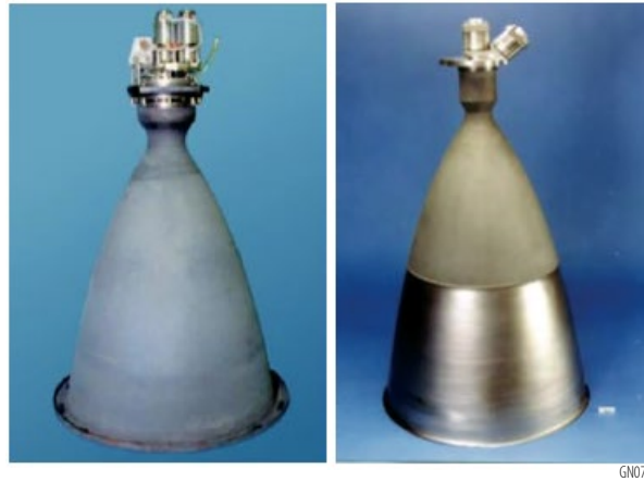
Figure B3-6: R-40B 4,000N and R-4D-15 450N (HiPAT) rocket engines (not to scale).
