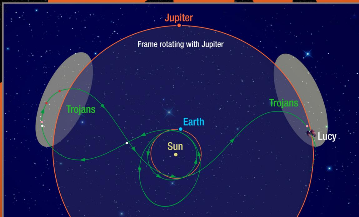
This diagram illustrates Lucy's orbital path. The spacecraft's path (green) is shown in a rotating view where Jupiter appears to stand still, giving the trajectory its pretzel-like shape.
