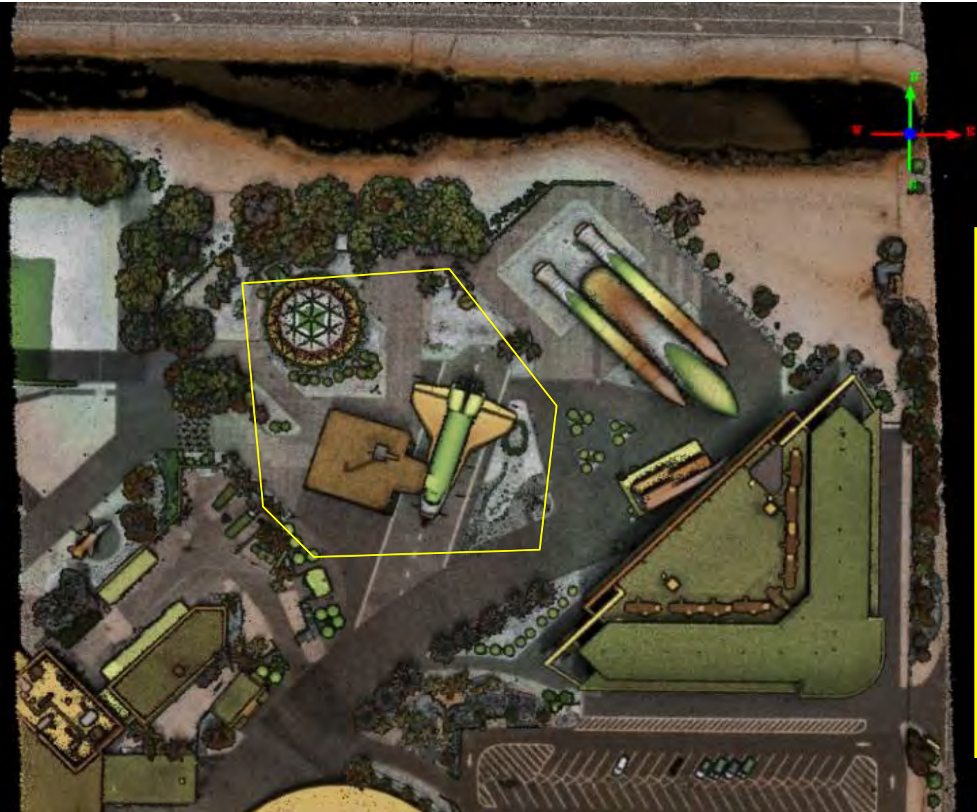
Lidar Point Cloud at 5cm post-spacing Color Coding by Z Coordinate & Intensity
