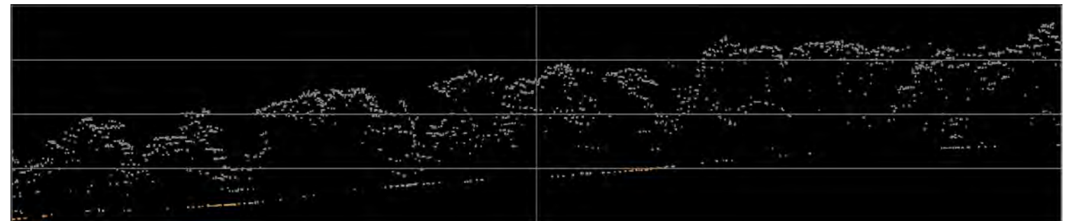
Leica ALS70 7,000 ft AGL 2PPSM Leaf On
