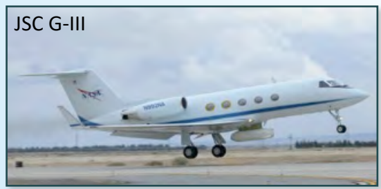
Non-pressurized pod with air inlets for cooling the radar electronics
