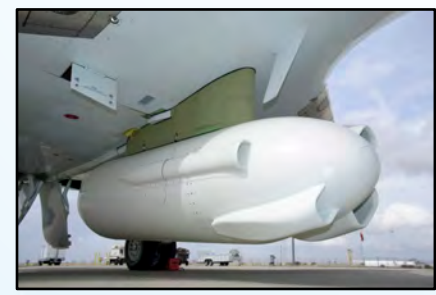
Non-pressurized pod with air inlets for cooling the radar electronics
