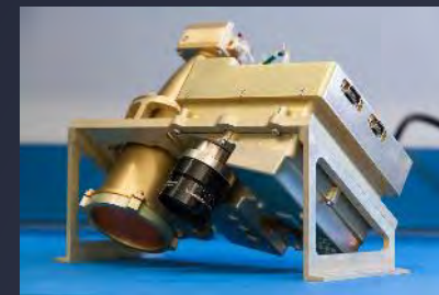
Near-InfraRed Volatile Spectrometer System (NIRVSS): Detects presence of H 2 O/OH as a function of illumination, surface temperature, and local time of day
