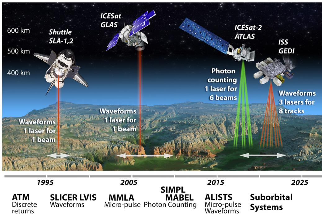
**FIGURE 9-3.** Profile sampling patterns for NASA Earth and planetary lidars. ICESat-2's six profiles are composed of profile pairs separated by 90 m to determine local slopes, with the pairs separated by 2 km. GEDI's eight profiles are separated by 600 m to sample terrestrial ecosystems uniformly. The starting dates of operations for these missions progress from left to right.
