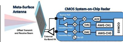
Block diagram of the CMOS SoC radar chip with the meta-surface antenna.
