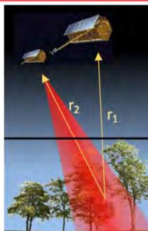
PolInSAR involves 2 or more satellites with specified polarization. Different baselines, polarizations, and radar frequencies, along with diverse scatterer characteristics will be simulated in OSSEs.
