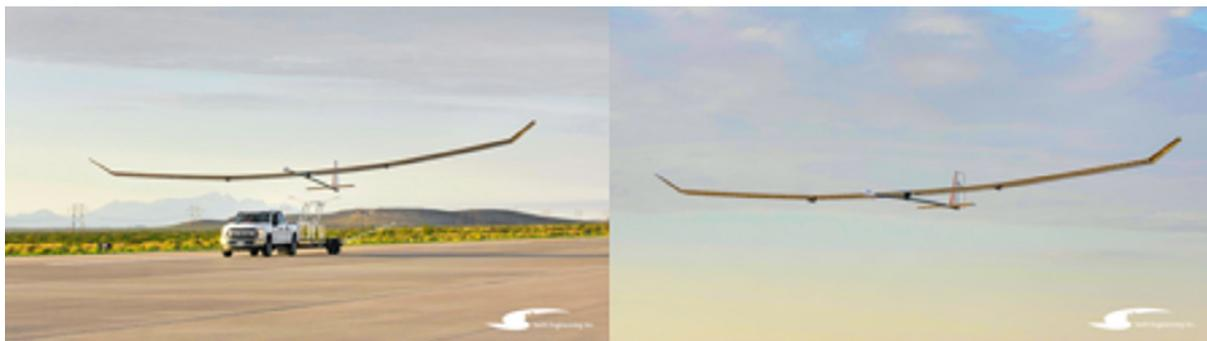
Aerovironment's HAPSMobile Sun glider (a joint venture with Softbank) recently completed low altitude test flights (Figure 9-7). This 260-ft wingspan HALE has a 6-month endurance and payload capacity of about 100 lb, and is designed to carry telecommunications equipment to provide better communications to under-served areas, including rural communities.
