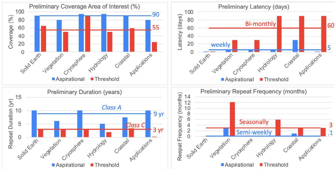
**FIGURE 8-3.** Instrument needs. For the resolution blue bars show aspirational needs and red threshold. Bars show median values across the disciplines with values noted.
