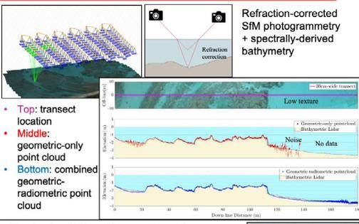
Refraction-corrected SfM photogrammetry + spectrally-derived bathymetry
