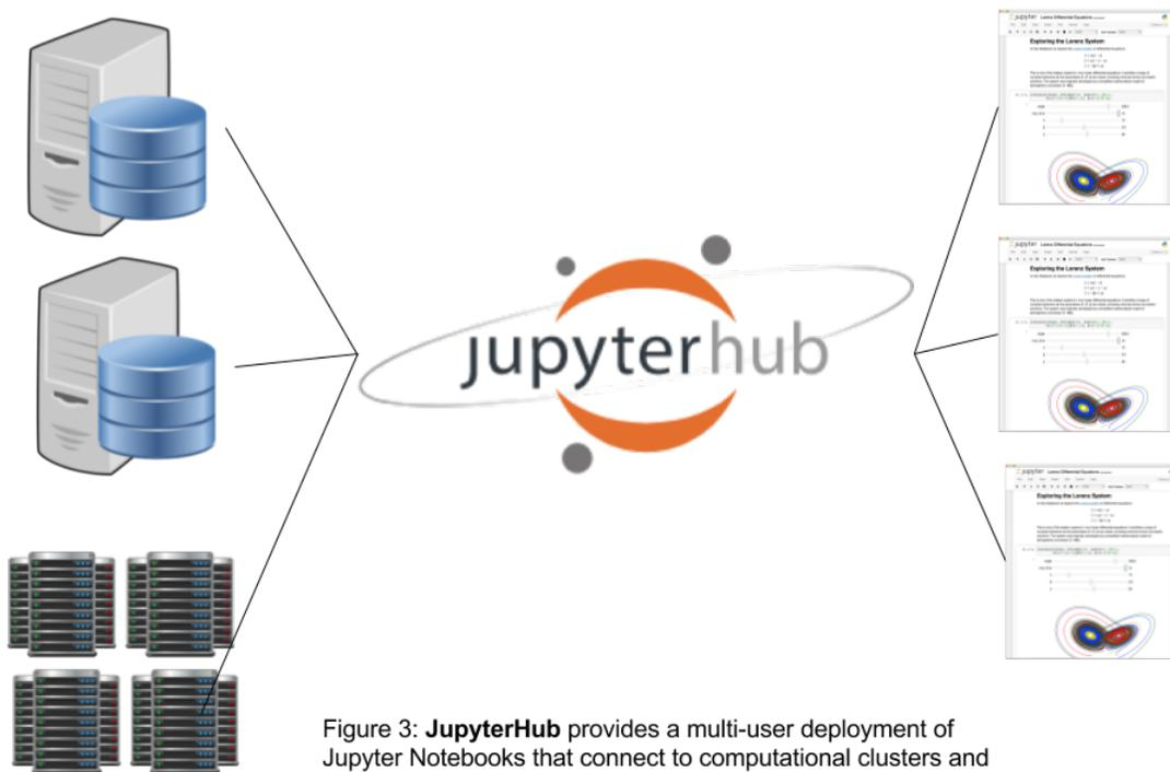
Figure 3: **JupyterHub** provides a multi-user deployment of Jupyter Notebooks that connect to computational clusters and shared databases, allowing for scaling up analysis capabilities
