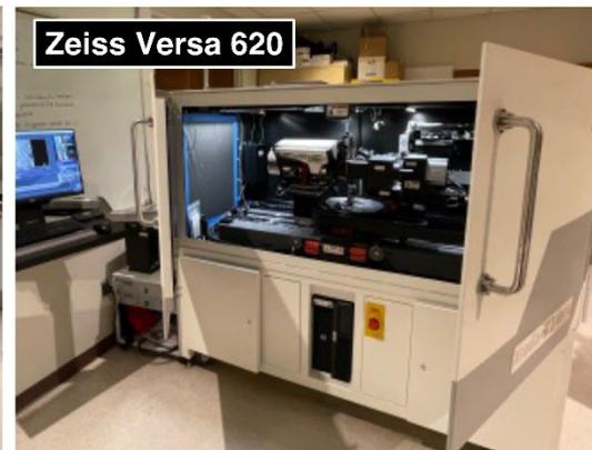
**UTCT XCT Scanners.** (left) NSI scanner: 450- and 225-kV X-ray sources and a flat-panel detector for larger and/or relatively more attenuating samples. (right) Zeiss Versa 620 scanner: 160-kV X-ray source and six detectors for smaller and/or relatively less attenuating samples and DCT.
